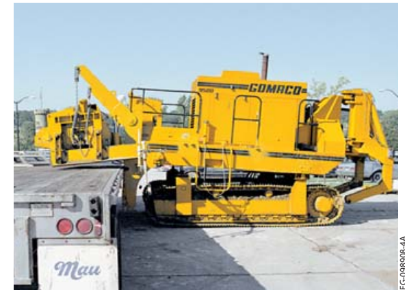
Optional hydraulic front lifting arms assist in the ease of loading the trimmerhead or receiving hopper onto the trailer for transport or positioning when mounting.
