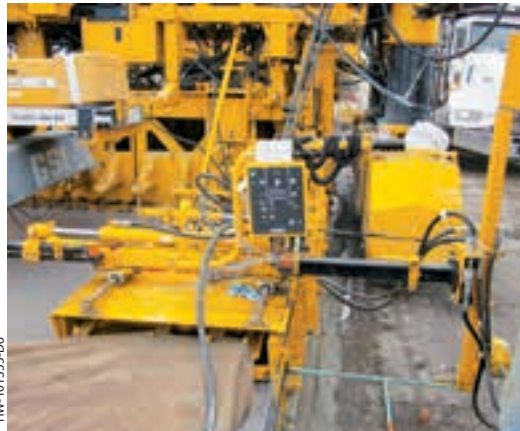
The 5400 series bar inserter is front or rear loading and front inserting for ease of use. It mounts to the mold's T-bar and allows on-the-go crown changes, while maintaining a constant depth. The bar box is mounted to the paver's rear T-beam mounting rail for easy access and loading of the bar magazine. There are individual depth guides on the right and the left side of the bar inserter in order to keep bars parallel to the top of slab. The 5400 series bar inserter can hold up to 50 bars in the bar magazine and bar loading chain system.
