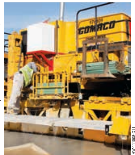
The 5400 series bar inserter is front or rear loading and front inserting for ease of use. It mounts to the mold's T-bar and allows on-the-go crown changes, while maintaining a constant depth. The bar box is mounted to the paver's rear T-beam mounting rail for easy access and loading of the bar magazine. There are individual depth guides on the right and the left side of the bar inserter in order to keep bars parallel to the top of slab. The 5400 series bar inserter can hold up to 50 bars in the bar magazine and bar loading chain system.
