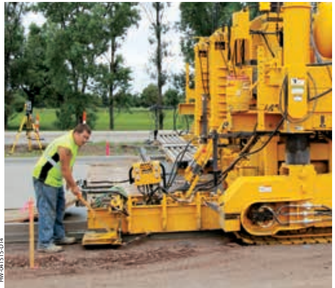
The trailing form with manual or air-powered bar insertion is designed to trail the track on two-track pavers. This system will accommodate most types of bars.
