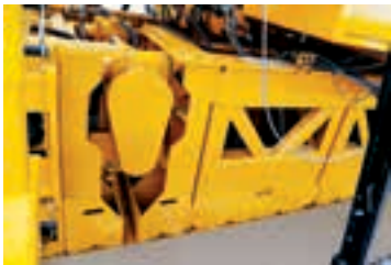
This 5400 series mold has a power transition adjuster (PTA) to provide on-the-go transitions in the crown of the concrete slab.
