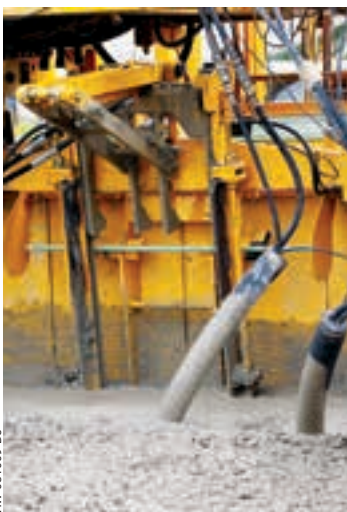
The 5400 series bar inserter is front or rear loading and front inserting for ease of use. It mounts to the mold's T-bar and allows on-the-go crown changes, while maintaining a constant depth. The bar box is mounted to the paver's rear T-beam mounting rail for easy access and loading of the bar magazine. There are individual depth guides on the right and the left side of the bar inserter in order to keep bars parallel to the top of slab. The 5400 series bar inserter can hold up to 50 bars in the bar magazine and bar loading chain system.
