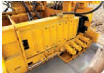
The telescoping end section of the 5400 series mold can include integral curb.
