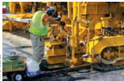
GOMACO's sideplate extension with the hydraulic system bar inserter.
