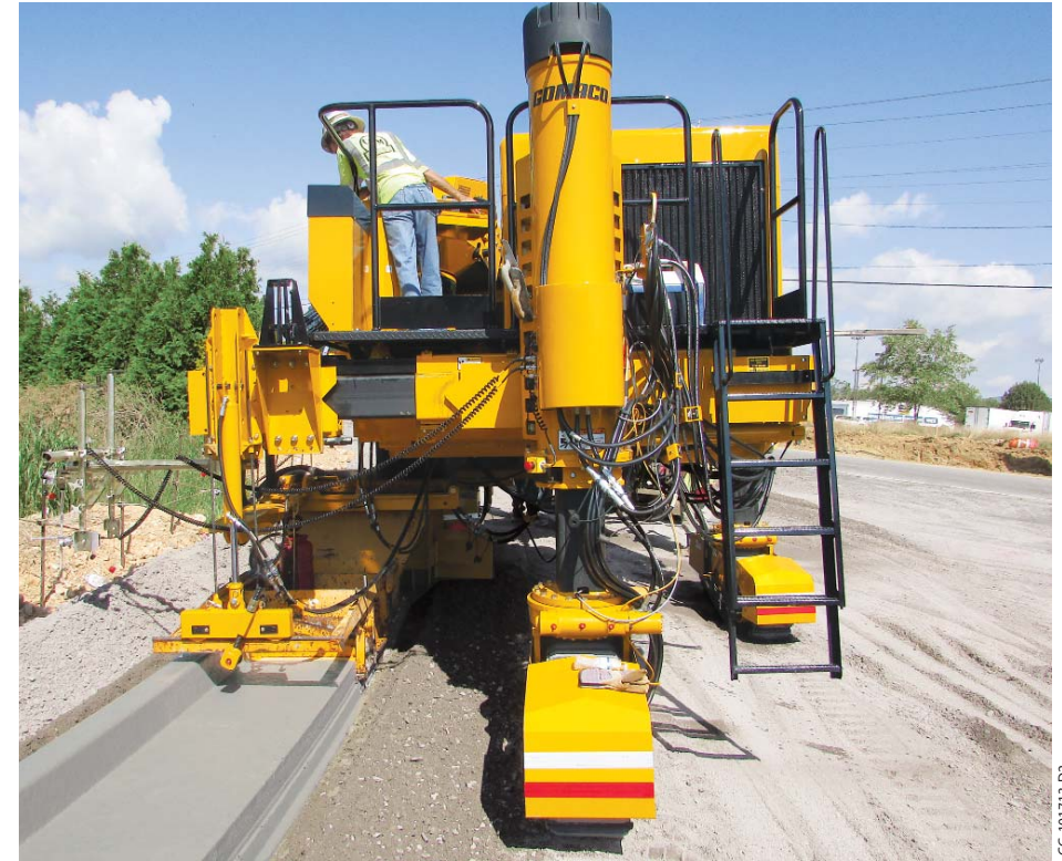
Intelligent All-Track Positioning (ATP) on the GOMACO Commander IIIx includes a smart hydraulic cylinder on each of the three legs. The smart cylinders allow G+ to know the position of all three tracks and make steering adjustments as needed.
