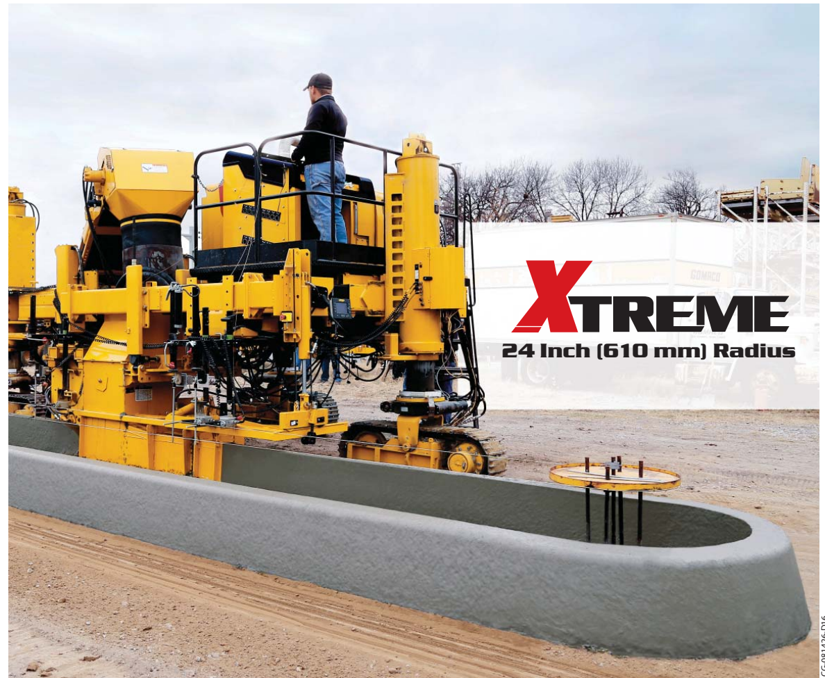
Contractors can now pave a 24 inch (610 mm) radius with the GOMACO Commander IIIx and G+ control system on stringline or 3D guidance system.
