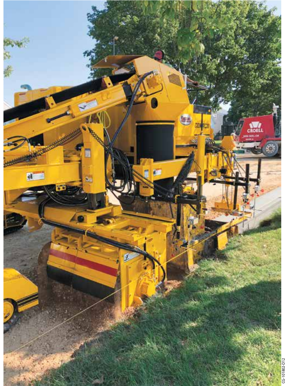
The three-track Commander IIIx has the ability to simultaneously trim the grade and slipform curb and gutter with ease.
