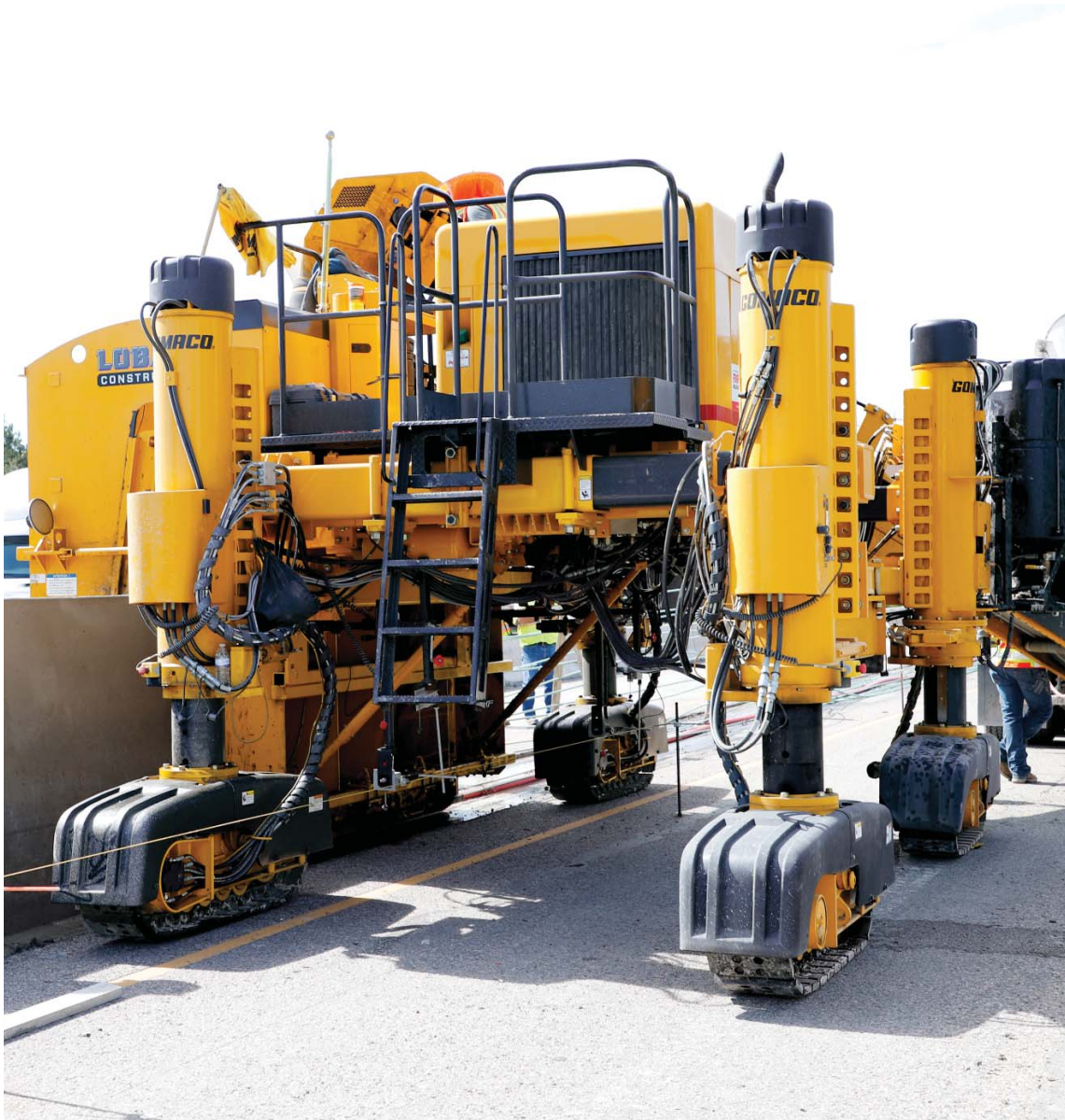
A five foot (1.52 m) variable barrier is being slipformed by the four-track GOMACO Commander III. It is equipped with a sidemounted mold and the four-track barrier package. The Commander III features a pivoting operator's console allowing the operator to have hands-on control and a clear view of the paving operation.
