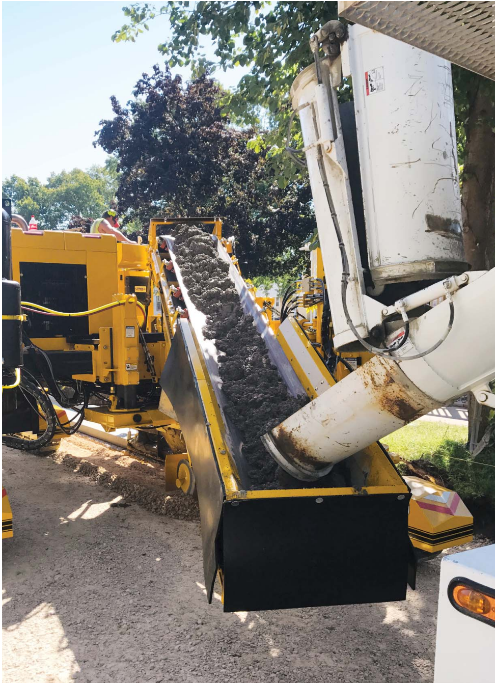
The conveyor on the Commander III has a length of 17.1 feet (5.21 m) and a width of 24 inches (610 mm) to allow for continuous concrete flow to the hopper.
