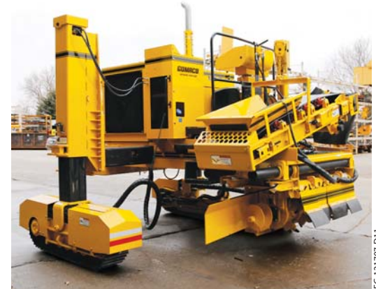
The Commander II has a minimum height of 7.4 feet (2.26 m) with the leg retracted, and a maximum height of 9.9 feet (3.02 m) with the leg extended.
