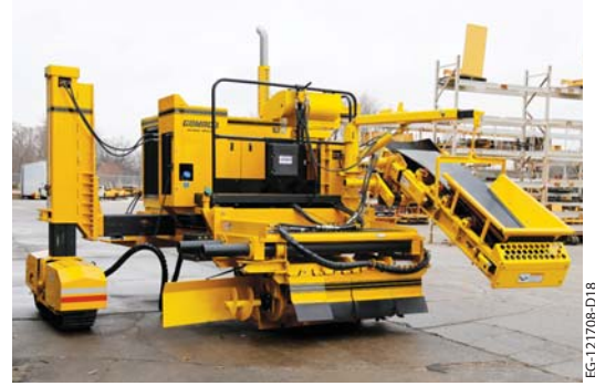
The right telescoping leg has a hydraulic side adjustment of up to 30 inches (762 mm).
