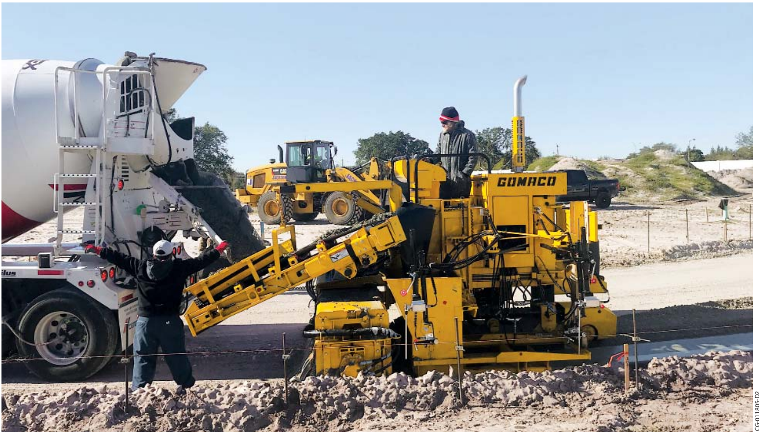
Operator comfort and visibility has been designed into the new Commander II. The operator's platform is isolated to eliminate vibration for operator comfort during paving.
