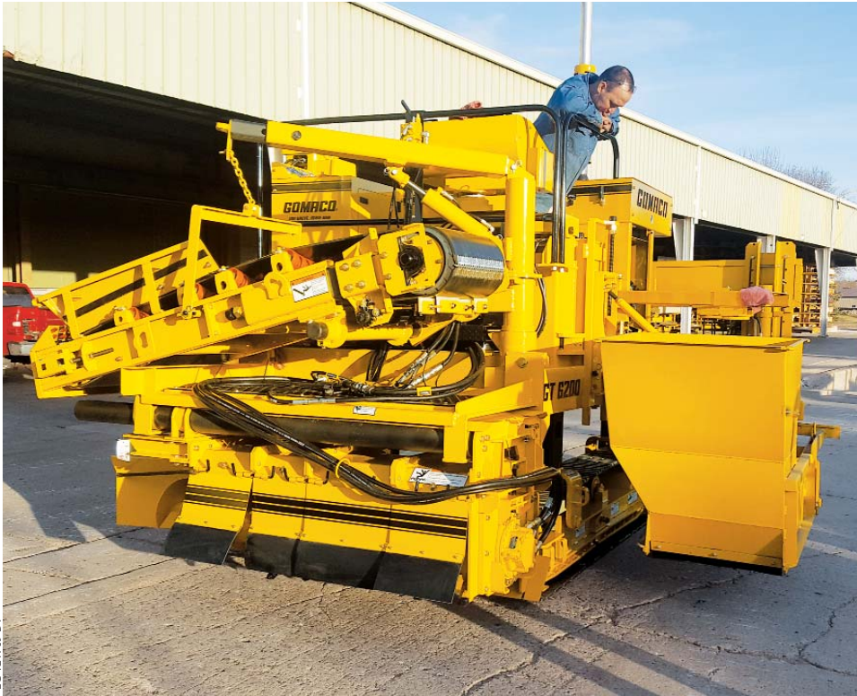
GOMACO's Commander II is equipped with a 60 inch (1524 mm) trimmerhead with sideshifting capabilities up to 48 inches (1219 mm).
