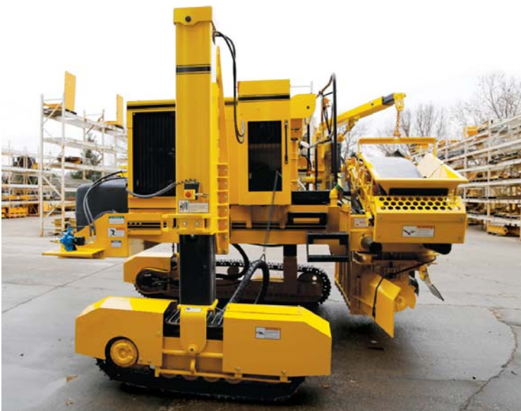
Commander II's right track has a hydraulic height adjustment of 30 inches (762 mm) and a manual height adjustment of 16 inches (406 mm). The left track has a hydraulic height adjustment of 20 inches (508 mm).
